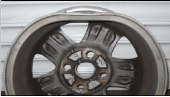
Fig. 2: Bend due to impact:
