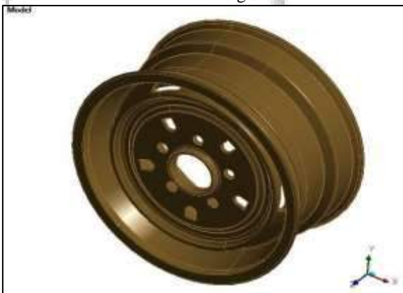
Fig. 3: Al Wheel rim CAD model in CATIA
