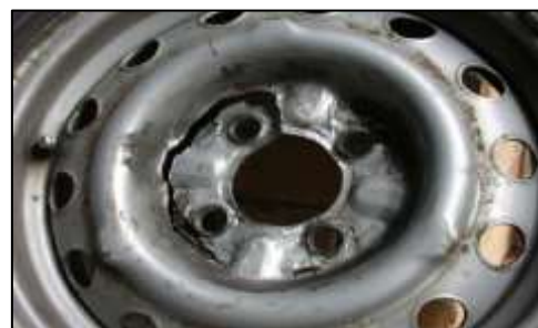
Fig. 1: Crack near the hub hole
