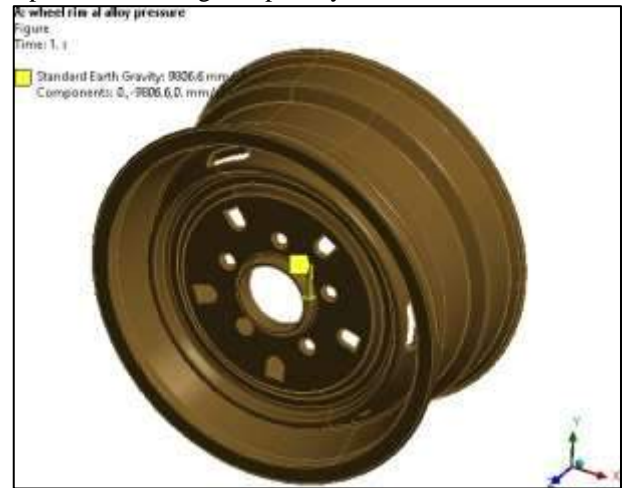
Boundary conditions for baseline wheel rim model
